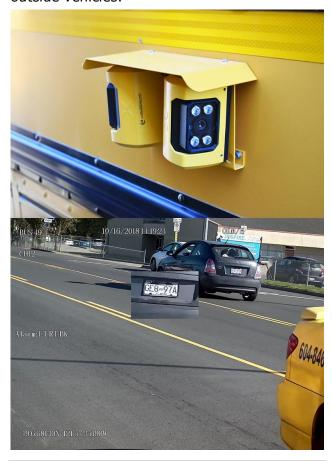
Gatekeeper's technology is able to capture license plates of vehicles in lanes 2, 3, and 4 with high, with its latest 10 megapixel stop arm camera system.
