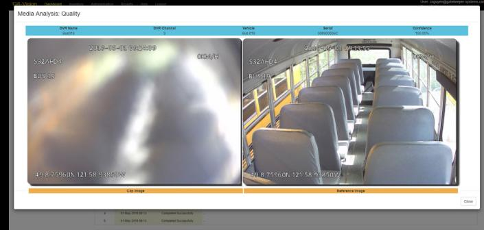
Figure 1 on the left shows a camera lens that has been vandalized with petroleum jelly vs the one on the right showing normal lens.
