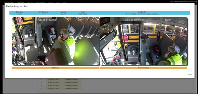
Figure 2 on the left shows a camera aim has changed as opposed to the image on the right where the aim has not been manipulated. Health Check will report such issues on the dashboard.
