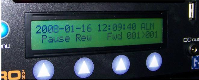
The system will display all Driver Alarm events. Time of the current alarm event occurs at the top of the LCD. Use the Fourth blue button, (as indicated), to navigate through the Alarm events. The default direction is forward, indicated by ">". Press "Rew" or "Fwd" to change the navigation direction. Choose the alarm you want and press the "Pause" button.
