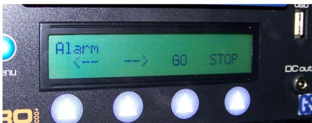
We can program the system to Mark and Save a segment of video. There are a few ways to do this. An easy solution is to search the video by the Driver Alarm events. Each event corresponds to a button press on the SmartFlag Alarm button. To browse by Alarm, press the button below the left pointing arrow until the LCD displays Alarm. Then press GO to browse the Driver Alarm signals saved on the unit.
