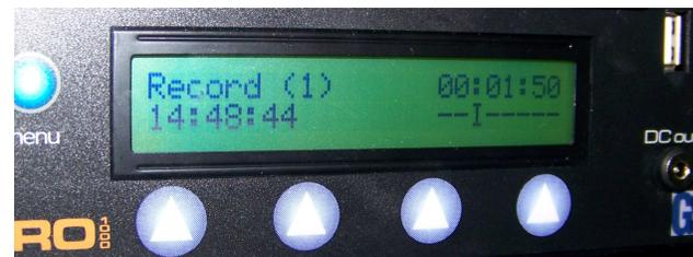
Press the Blue Menu button until the Playback option is displayed and then press the button beneath GO.
