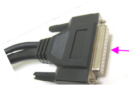
Existing Power Harness Connector
