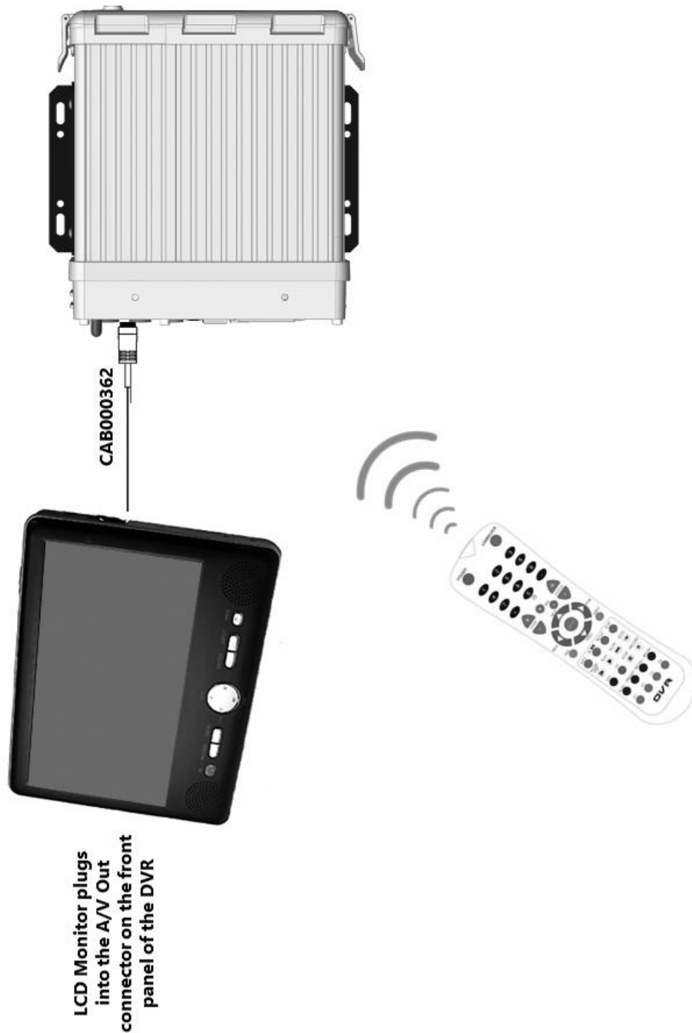
Figure 3-2 Connecting the IR Remote Control and LCD Monitor
