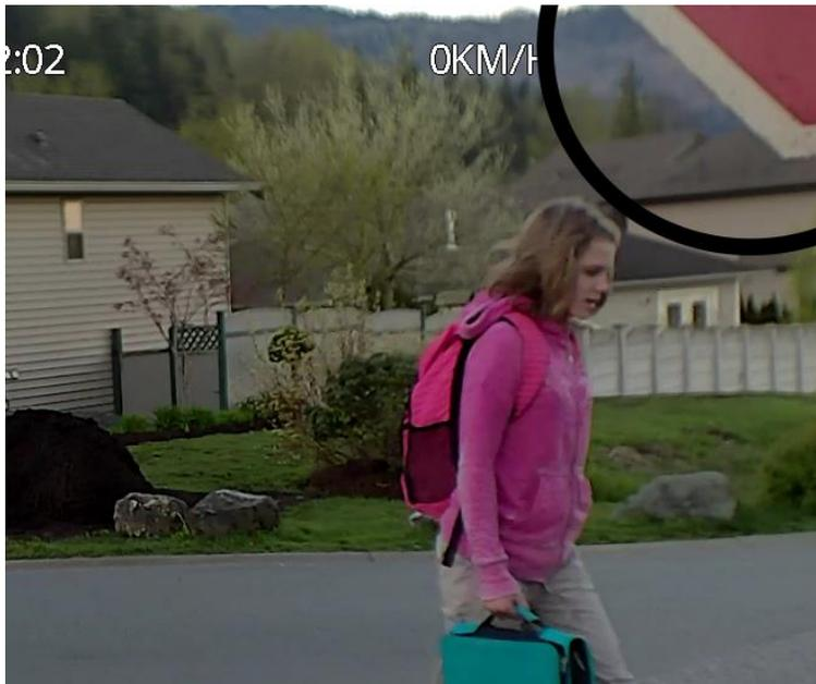
**Figure 2.** Camera mounted so deployed stop arm is visible in top right corner of image
