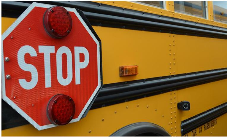
**Figure 1.** Camera mounted 54 inches behind stop arm base and between rub rails
