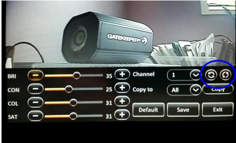
Select the camera by clicking on the arrow next to the Channel button. Use the two view orientation buttons (in the blue oval) to change the image to the required orientation and click SAVE and then EXIT. Normally it is necessary to do both a vertical and horizontal flip to get the image to be in the proper orientation. Ensure desired image is what is on the screen.
