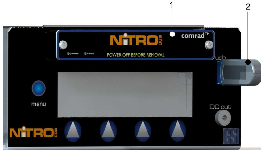
Using an Gatekeeper Systems Inc. approved USB flash drive to repair a corrupt COMRAD™
